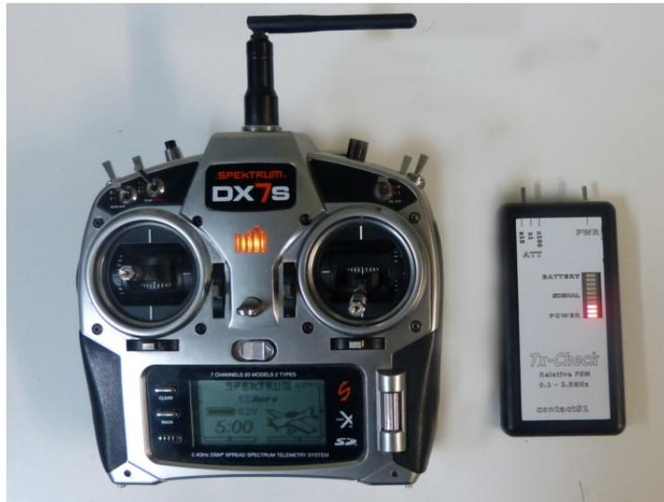
Depicted here is the Tx-Check measuring the output of a suspected faulty transmitter. When the transmitter was new and known to be working well, when placed in this position and proximity to the Tx-Check RFSM the indication on the bar graph display was 4 bars. As seen here 3 bars are lit indicating that the transmitter is outputting less RF power now than when known good. The RF power module in the transmitter was replaced and power restored to its known good state.
